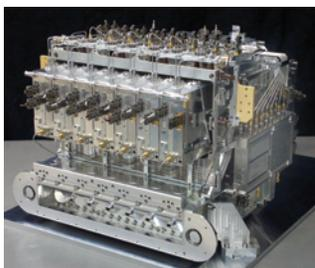
L'instrument Heterodyne Instrument for Far-Infrared - HIFI emploie la technologie des diodes supraconductrices. / The Heterodyne Instrument for Far-Infrared (HIFI) employs superconductor diode technology.
